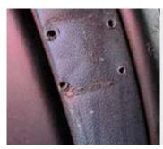
Deep scratches or marks on the instrument panel. Drill holes in the dashboard. Missing cover plates.
