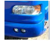
Surface scratches on the combi-light due to daily use. Combi-light unit is clear, no condensation and dirt is not able to penetrate.
