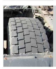
Normal wear in the carcass of the tyre and NO punctures in the profile.
