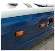
Cracks and fracture in side skirts.
