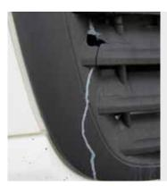
Damage and cracks on grille.
