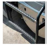
Surface scratches on stairs to catwalk.
