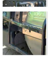
Deformed or bent stairs.
