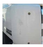
Cracks and fracture on the outside of the air deflectors.
