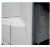
Cracks and fracture on drivers and passengers doors.
