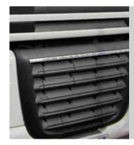
Minor damage due to stone chippings.
