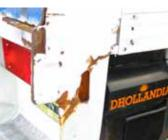
Corner of body work dented and loading edge bent.
