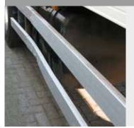
Bent or distorted under runs, including associated support.
